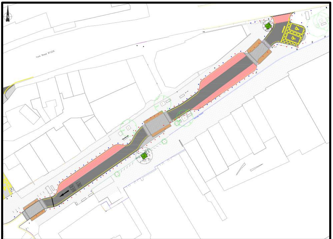
Fig 5 – Initial review of bollards (red dots might be removed, blue dots might stay)
